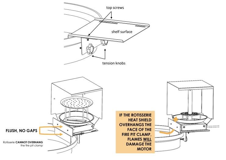
ANY GAP PRESENT WILL VOID WARRANTY AND COULD RESULT IN FAILURE OF DEVICE
